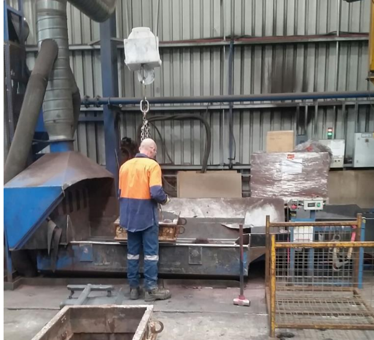
Figure 12 Shakeout of sand involves electricity for vibration and extraction
