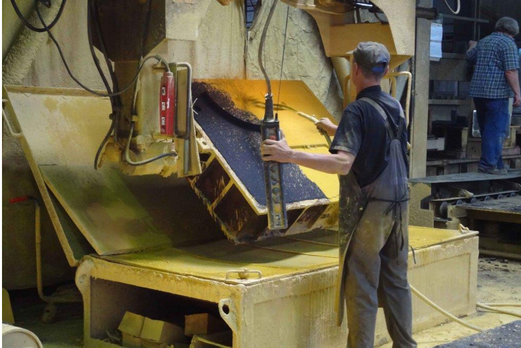
Figure 14 Mould preparation involves mixing, compression and heat
