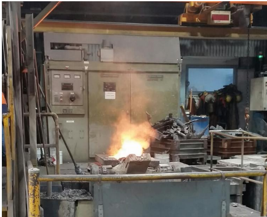
Figure 11 Casting involves electricity for heat and fume extraction
